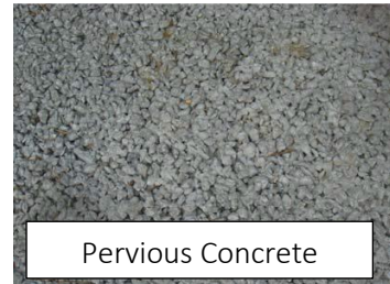
Figure 7.2: Permeable Pavement Examples
